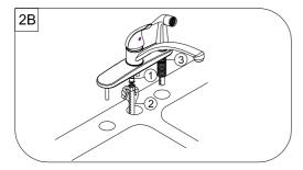
For Models with an Integral Spray Support (Fits 3-hole sinks) Place new faucet in position on the sink.Insert spray hose (2)down through spray support (3) on escutcheon and far right hole in sink.Insert spray hose up through center hole in sink.Attach spray hose (2)to spray hose nipple (1).
