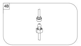
(B) Ball Nose Flexible Supplies: If you are using ball-nose flexible supplies to connect the faucet to water supply lines: Slip coupling nut behind ball-nose of flexible supply tube. Ball nose coupling will go partially into IPS shank or fitting. Tighten coupling nut (DO NOT OVER TIGHTEN). Install opposite end according to manufacturer's instructions for both tubes.
