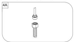
(A) Stainless Steel Braided Faucet Supply Tubes: This is the simplest of all installations. If you are using stainless steel braided faucet supply tubes, this faucet requires one end of the supply tube to have a 1/2" female IPS connection. The other end of this supply tube must match the thread on the water supply fittings or shut off valve under your sink. Once you have identified the required tube, carefully follow the manufacturer's installations instructions for each tube
