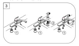
From under sink, threads mounting nuts (1) onto faucet. Tighten mounting nuts. screw locknuts (2) onto threaded shanks and hand tighten.
