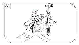
For Models with a Spray Support (Fits 4-hole sinks)
