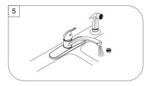
Remove AERATOR and turn faucet handle all the way on. Turn on hot and cold water supplies and flush water lines for one minute.
