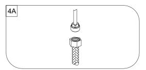
(A) Stainless Steel Braided Faucet Supply Tubes: This is the simplest of all installations. If you are using stainless steel braided faucet supply tubes, this faucet requires one end of the supply tube to have a 1/2" female IPS connection. The other end of this supply tube must match the thread on the water supply fittings or shut off valve under your sink. Once you have identified the required tube, carefully follow the manufacturer's installations instructions for each tube
