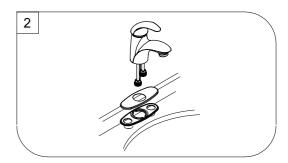
Place escutcheon and base plate on the sink. Position the new faucet through mounting hole.
