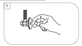
Shut off water supplies. Remove old faucet. Clean sink surface in preparation for new faucet.
