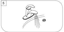
Remove AERATOR and turn faucet handle all the way on. Turn on hot and cold water supplies and flush water lines for one minute.
