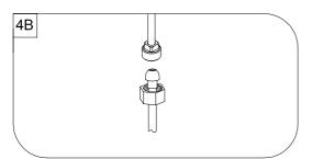
(B) Ball Nose Flexible Supplies: If you are using ball-nose flexible supplies to connect the faucet to water supply lines: Slip coupling nut behind ball-nose of flexible supply tube. Ball nose coupling will go partially into IPS shank or fitting. Tighten coupling nut (DO NOT OVER TIGHTEN). Install opposite end according to manufacturer's instructions
