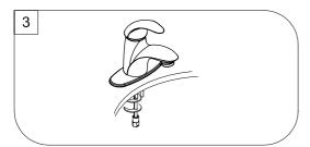
Screw the mounting stud into the body. Secure the faucet to sink by installing rubber washer, steel washer and nut onto it. Tighten with wrench.
