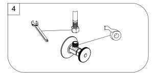
Apply pipe tape onto threads of water supplies.
