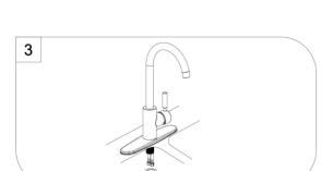
Screw the mounting stud into the body. Secure the faucet to sink by installing rubber washer, steel washer and nut onto it. Tighten with wrench.
