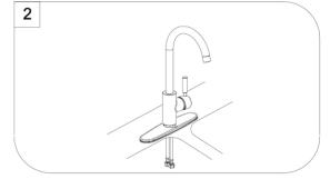
Place optional deckplate on bottom of new faucet before position faucet through mounting hole.
