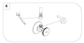
Apply pipe tape onto threads of water supplies. Use wrench when tightening the hose connection, do not overtighten.
