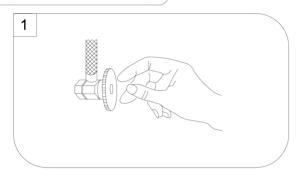
Shut off water supplies. Remove old faucet. Clean sink surface in preparation for the new faucet.
