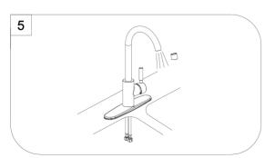
Important: After installation is completed. Turn on water supply and allow both hot and cold water to run for at least one minute each. While water is running, check for leaks. Reinstall Spray head. Your new faucet is now ready to use.
