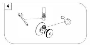
Apply tellon tape onto threads of water supplies. Use wrench when tightening the hose connection, do not overtighten.
