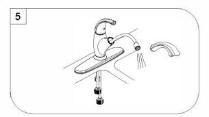
Important: After installation is completed. Turn on water supply and allow both hot and cold water to run for at least one minute each. While water is running, check for leaks.
