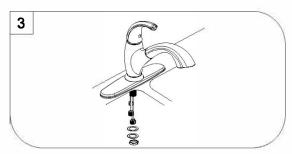
Secure the faucet to sink by installing plastic washer steel washer and nut onto it. Tighten with wrench.
