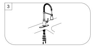
Remove the 2 screws from locking nut .From under the sink,install the rubber washer,steel washer,and locking nut onto the shank Tighten the locking nut with a basin wrench or socket tool and install the 2 screws to secure the faucet in place.
