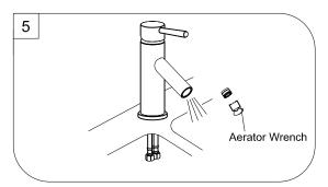
Important: After installation is completed. Remove aerator then turn on water supply and allow both hot and cold water to run for at least one minute each. While water is running, check for leaks
