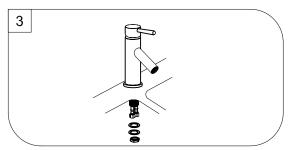
Screw the mounting stud into the body. Secure the faucet to sink by installing plastic washer , steel washer and nut onto it. Tighten with wrench.
